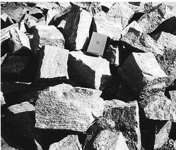
Fig. 12.2 Dimension stones (gneissic granite) piled up for engineering construction
