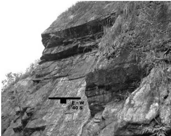
Fig. 3.17 Joints in quartzite depicting a bedding joint or dip joint with strike E–W dip 40^\circ South
