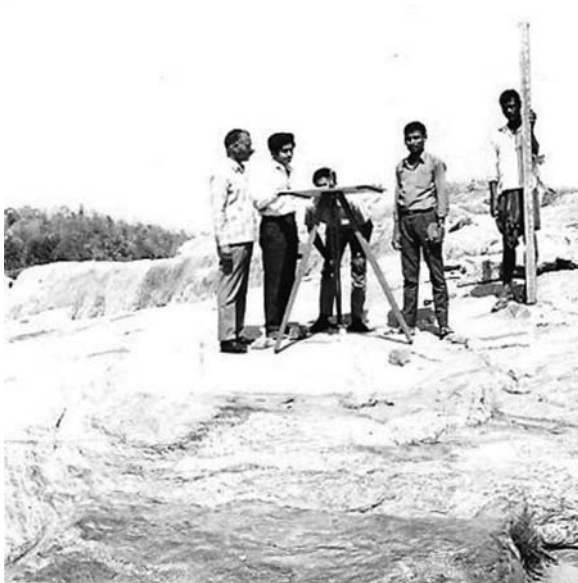
Fig. 11.6 Plane table mapping of a project site
