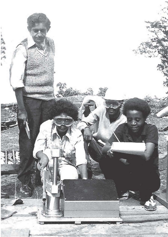
Fig. 10.1 Determining the strength of intact rock by point load testing machine
