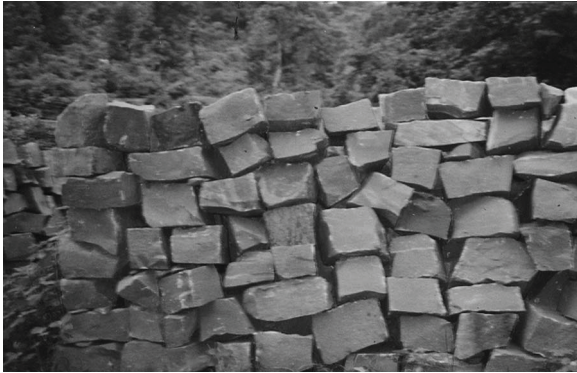
Fig.12.3 Dressed blocks of Vindhyan sandstone widely used in constructing ancient buildings and other masonry works
