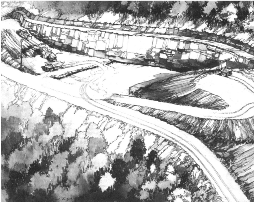
Fig. 14.3.0.2. Conventional haulback mining utilizing trucks, dozers, and front-end loaders. (Anon., 1979; illustration by Frank Kulczak. By permission from Skelly and Loy, Harrisburg, PA.)
