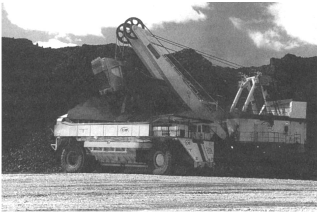
Fig. 14.3.2.6. Production face: 40-yd 3 (30.6-m 3 ) shovel loading 170-ton (154-t) bottom-dump truck.
