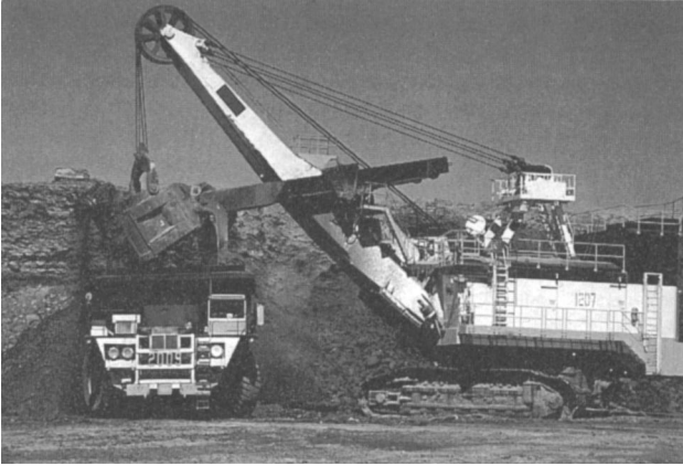
Fig. 14.3.2.5. Stripping operations: 36-yd 3 (27.5m 3 ) shovel loading 170-ton (154-t) end-dump truck.
