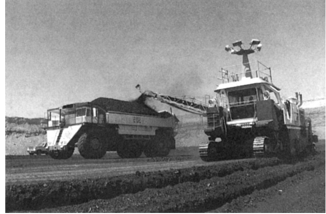
Fig. 14.3.2.7. Continuous-miner loading a 170-ton (154-t) bottom-dump truck.
