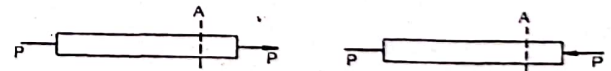
Fig. A rod of cross-section A subjected to a force P (left) tensile (right) compressive.
