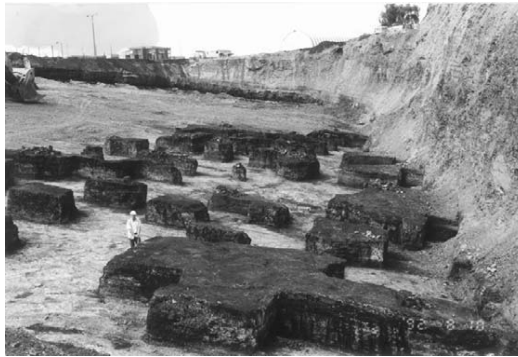
Figure 2.1a Old pillared workings in coal exposed at the Tinsley Park opencast site, Sheffield, England.
