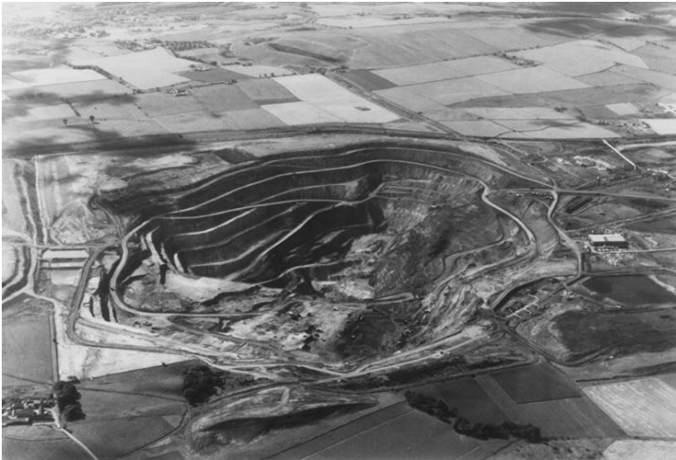
Figure 6.23b Restoration of the Westfield Opencast workings for coal, UK. The area beyond the current opencast workings has been rehabilitated and restored to agricultural land.
