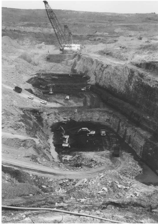
Figure 6.8 Opencast working of coal at St Aiden's opencast site, Yorkshire, England, with partly restored area at the top of the photograph.
