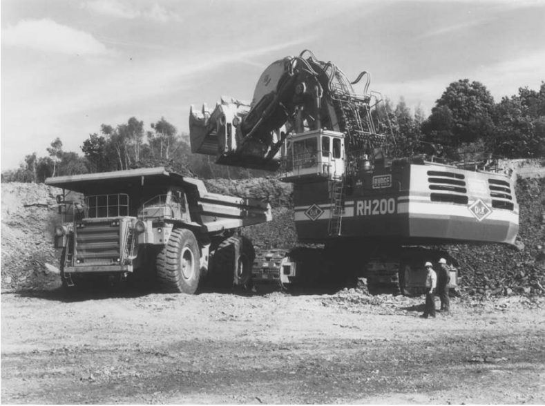
Figure 6.6 A dump truck being loaded by an electrically operated shovel. (Reproduced by kind permission of International Mining Consultants Limited.)
