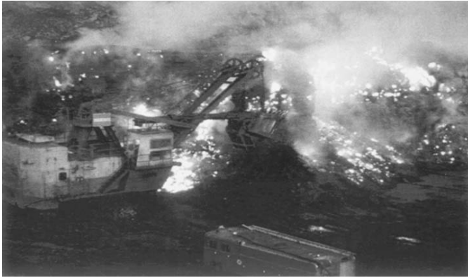
Figure 10.4 Fires caused by spontaneous combustion of coal in an opencast mine, Singrauli Coalfield, India. (Reproduced by kind permission of International Mining Consultants Limited.)
