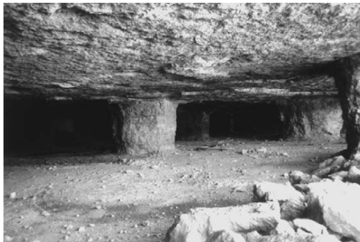
Figure 2.1b Old pillar working in the Bethaney Falls Limestone, greater Kansas City, United States.
