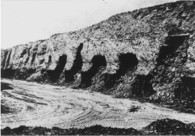
Figure 2.11 Void migration above a coal seam exposed by opencast workings in Staffordshire, England.
