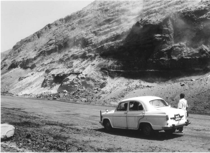
Figure 6.9 Pillars of coal left to retain overburden, Jayant Opencast Mine, Singrauli Coalfield, India.
