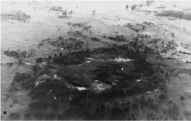
Figure 7.1 A colliery spoil heap in the Witbank Coalfield, South Africa, from which coal has been partially recovered and which shows signs of having been burnt.
