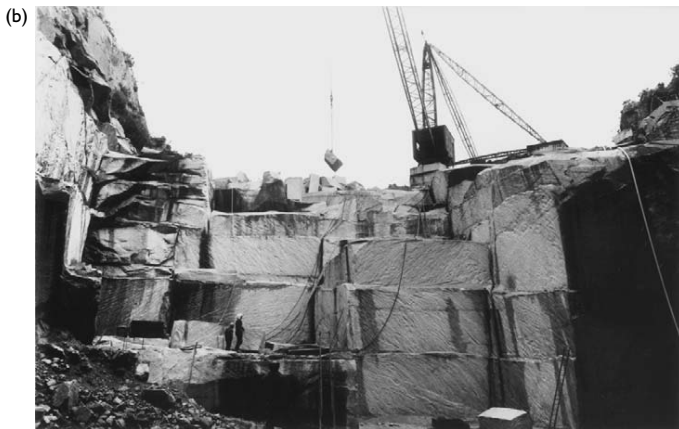
Figure 6.3 (a) Extraction of marble by diamond impregnated saw at Estremos, Portugal. (b) Working granite with a flame torch in Cornwall, England.
