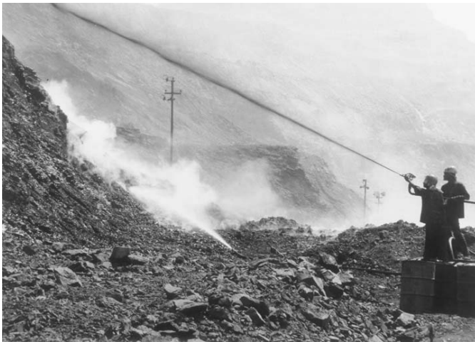
Figure 10.6 Extinguishing fires by water jetting and then spraying face with a bitumen compound at high pressure, Singrauli Coalfield, India.
