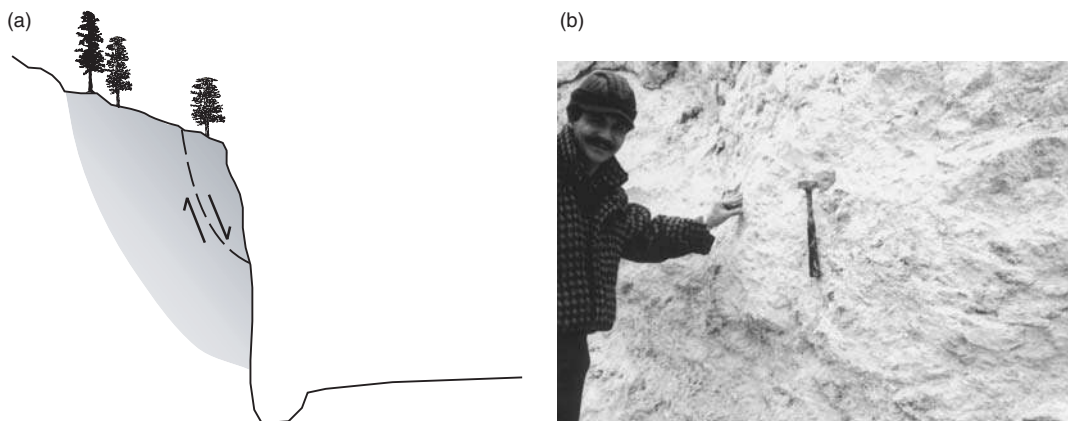
Figure 4.5 Shallow failure in very weak, massive rock containing no discontinuities (volcanic tuff, Trans European Highway, near Ankara, Turkey).
