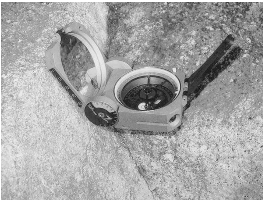
Figure 3.6 Geological compass (Clar type) used to directly measure dip and dip direction of surfaces. Lid is placed on surface and body is rotated until it is level, as indicated by the spirit level; the needle is released to indicate dip direction, and the dip is read off scale on the hinge. (The Brunton Co., Riverton, WY.)
