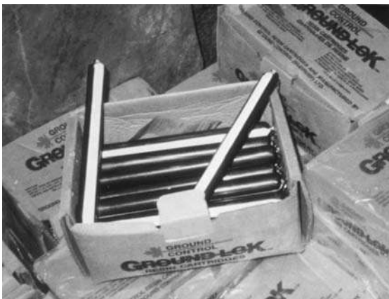
Figure 12.10 Resin cartridges for anchoring rock bolts (TRB, 1996).
