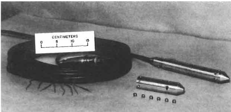
Figure 4.7 The USBM borehole deformation gauge.
