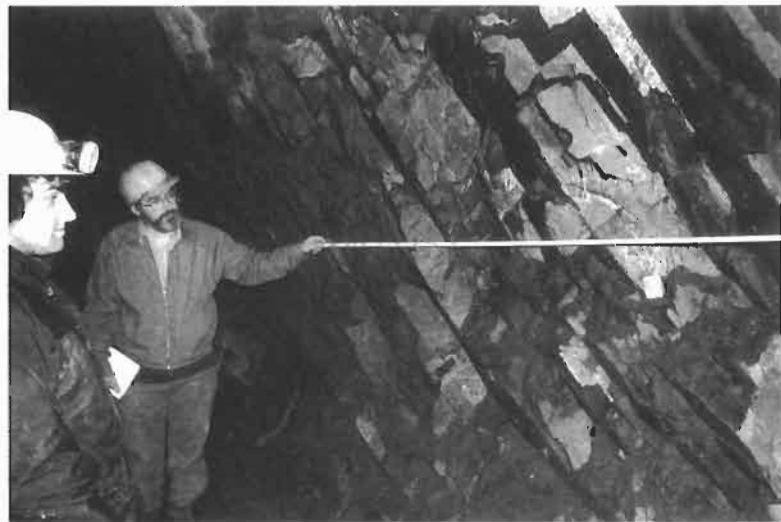
Figure 2.2 'Layered' intact rock.
