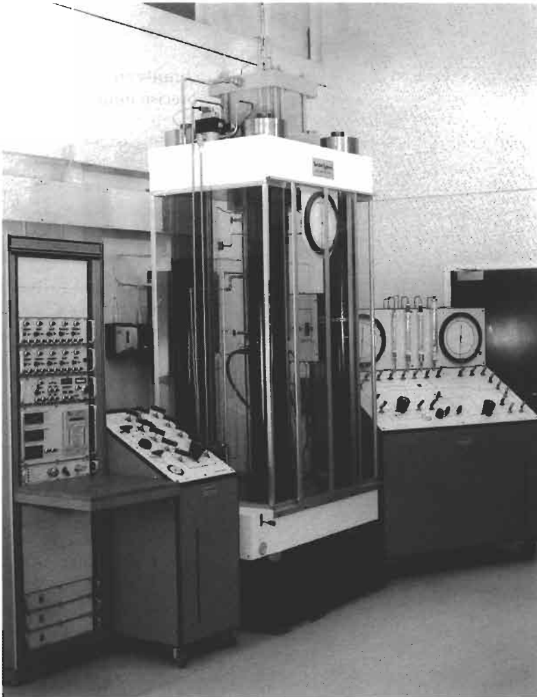
Figure 11.11 TerraTek servo-controlled triaxial testing machine at Imperial College as used for thermo-hydro-mechanical testing of discontinuities.
