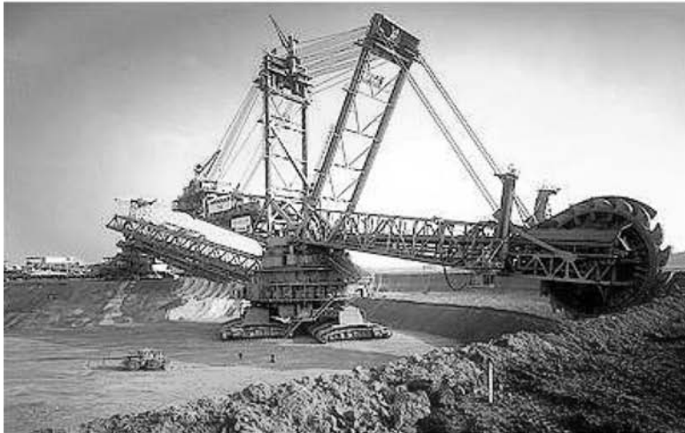
(b) Bucket wheel excavator – the largest mining equipment on earth. This technical giant is custom designed and built for the specific operating conditions and production rates. Currently attained and production rates are up to 240,000 m 3 (bank) per day, digging heights of as much as 100 m and service weights of 13,500 tons. (Courtesy: Krupp, 2000)
