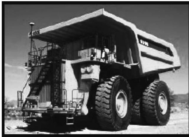
Figure 7.16 Giant sized 320 tons capacity trucks working at one of the surface coal mines in Australia.
