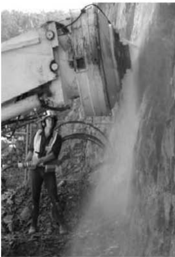
Figure 19.14 (a) Several mining companies are actively developing fully-autonomous surface drills. (b) It permits round design on-the-fly. (c) 'Oscillating Disc Cutting' – a novel technology for cutting hard rock at high rates with low cutter forces. 6
