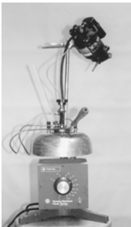
FIGURE 2.7 Pensky-Martens flashpoint tester.
