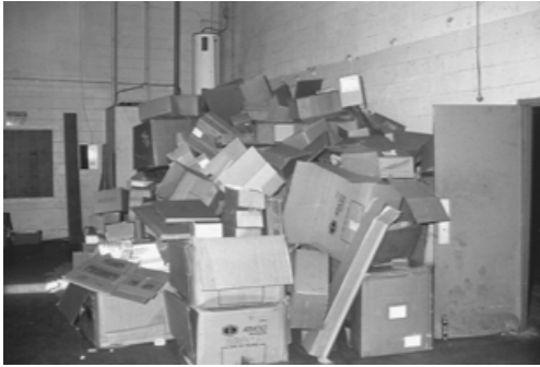
FIGURE 5.5 Accumulation of combustible material.
