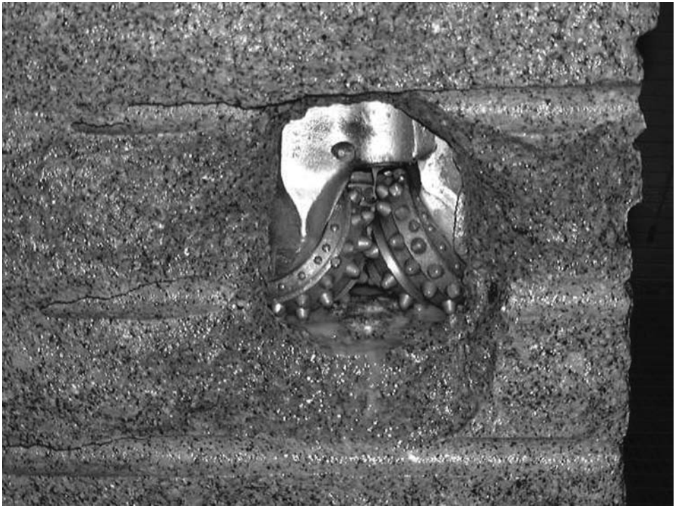
Figure 10.17. Cross-section through the hole of Figure 10.16 showing the bit and the cutters. Atlas Copco (2012a).
