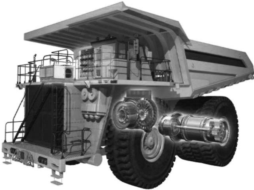
Figure 12.26b. Cutaway showing the propulsion system. Komatsu (2012).
