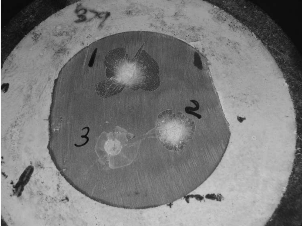
Figure 10.19. Plan view showing several isolated indentations made in a rock surface under laboratory conditions. Atlas Copco (2012a).
