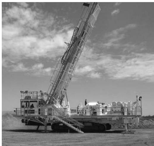
Figure 10.27. Sandvik D90KS drill rig with the mast positioned for drilling angled holes in an Australian mine. Sandvik (2012d).
