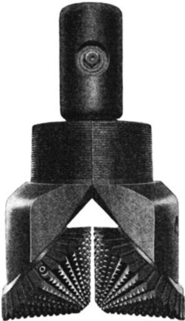
Figure 10.2. Frontal view of the Sharp & Hughes rock bit. Hughes (1916).
