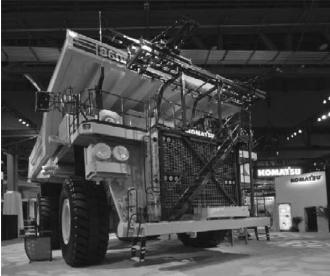
Figure 12.35. Trolley-equipped 860E truck. Komatsu (2008).
