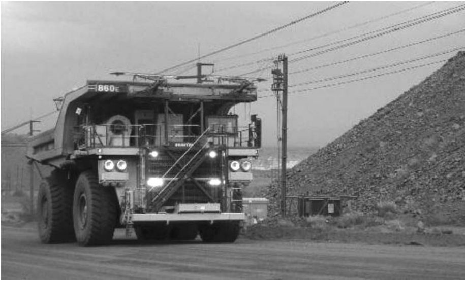
Figure 12.36. Truck operating under trolley power. Komatsu (2009a).
