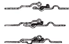
(a) PUSH-IN TYPE JOINT WITH INTERNAL RUBBER SEALING RING
