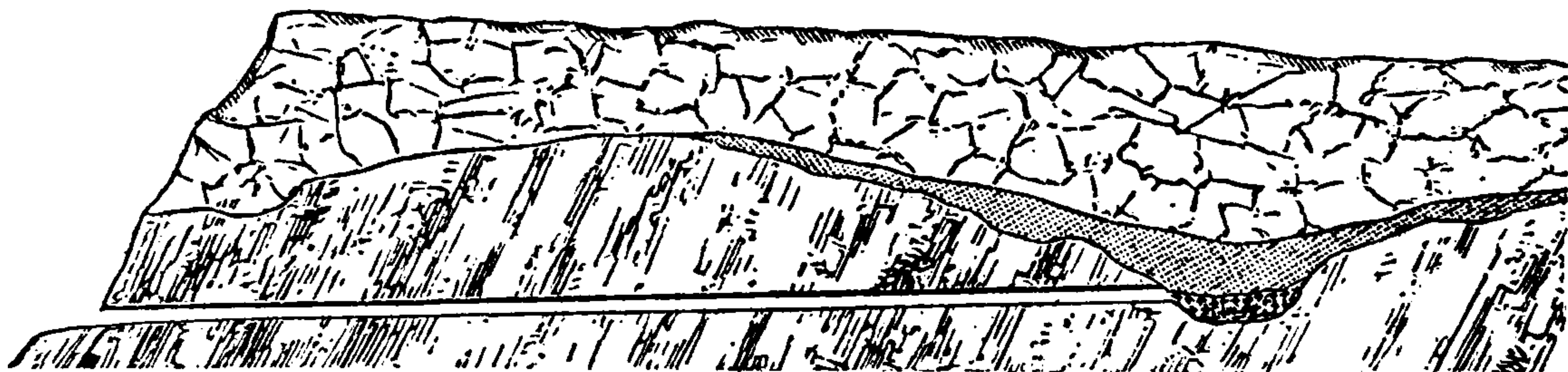
FIG. 10.—Section of Deep-Lead in Daylesford District, showing position of gold-bearing wash. (After R. B. Smyth.)
