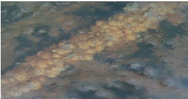
Fig. 4.5. A piece of straw under the dissecting microscope from the creek to which straw was added. Note the iron precipitates (mineral balls) on the straw. (Photographs by Boojum Research)
