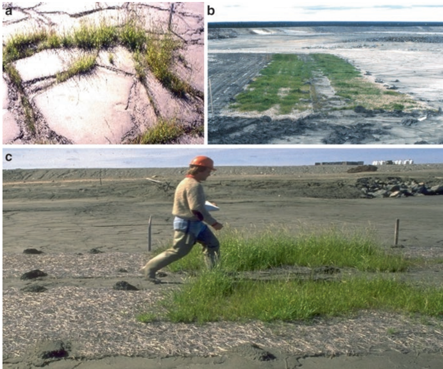
Fig. 9.15 Field experiments to grow grass and vegetation on fresh tailings. (a) Vegetation seeds were added to the fresh tailings spigot line. Results were not satisfactory, as vegetation only grew in the cracks. (b) The more satisfying efforts with straw mats and CPMW. (c) Boojum researcher, Martin Smith, monitoring the grass plots. (Photographs by Boojum Research)
