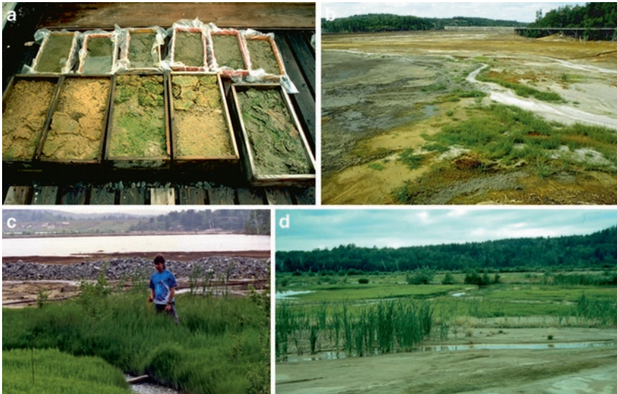
Fig. 4.3 Ecological engineering measures for stabilization and cover for pyrrhotite tailings. (a) Tailings covered with alkaline mine slimes fosters colonization by indigenous plants. (b) Experiments to fertilize the pyrrhotite tailings surface at various times during the season. Fall fertilization was successful. (c) Horsetails colonized the alkaline mine slimes without any fertilizer. In background are the permeable waste rock dikes to accumulate mine slimes. (d) Tailings several years after decommissioning recommendations implemented. (Photographs by Boojum Research)
