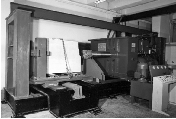
FIGURE 5.12 Horizontal drill rig in ITU laboratories.
