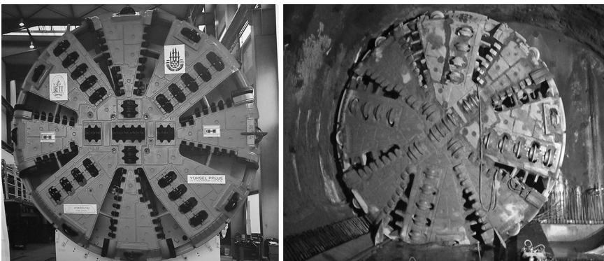
FIGURE 9.20 TBM S-360, cutter head with grill bars on the right and cutter head before modification on the left in Kozyatagi–Kadikoy (Istanbul) Metro Tunnel. (From archive of N. Bilgin.)
