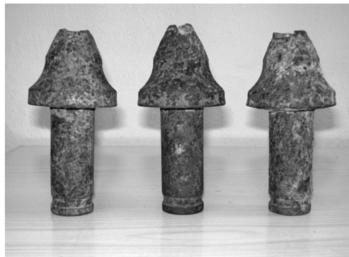
FIGURE 6.18 Breakage of the tungsten carbide tip due to a small amount of cobalt in high-strength andesite and limestone.
