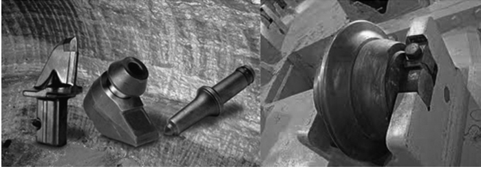
FIGURE 4.1 Radial cutters (left), conical cutters (middle), and disk cutters (right).
