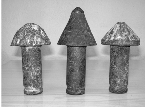
FIGURE 6.16 Symmetrical wear due to high abrasive characteristic of sandstone.
