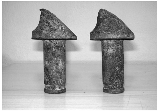
FIGURE 6.17 Asymmetrical wear due to malfunction of tool holder in siltstone and sandstone.
